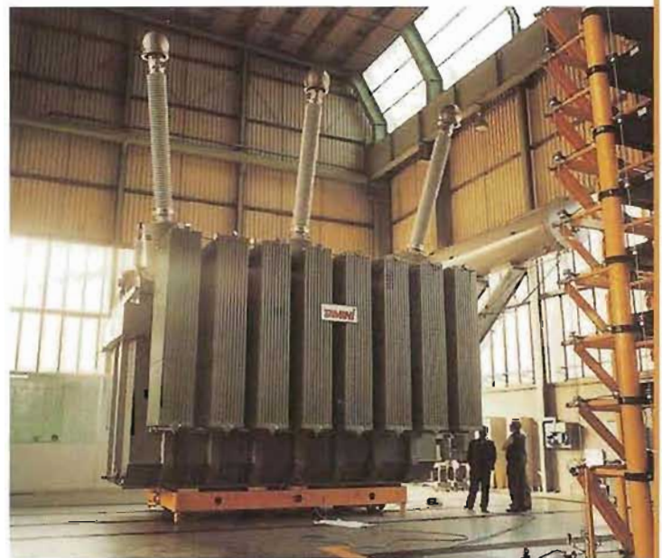
125 MVA - 250 kV power transformer for a substation in Switzerland during testing
