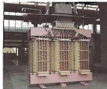
Internal view of one of 18 rectifier transformers, 26.8 MVA (Canada)
