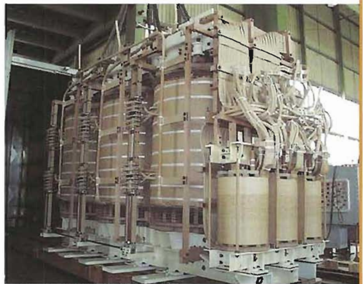
One of six autotransformers 240 MVA - 300/245/145 kV (UK)
