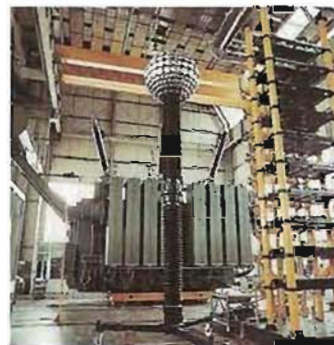
125 MVA - 250 kV power transformer for a substation in Switzerland during testing
